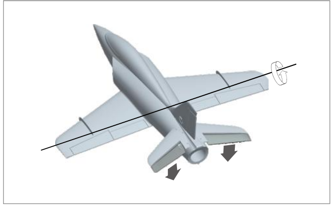
Nose up during flight—Elevator correction diagram
