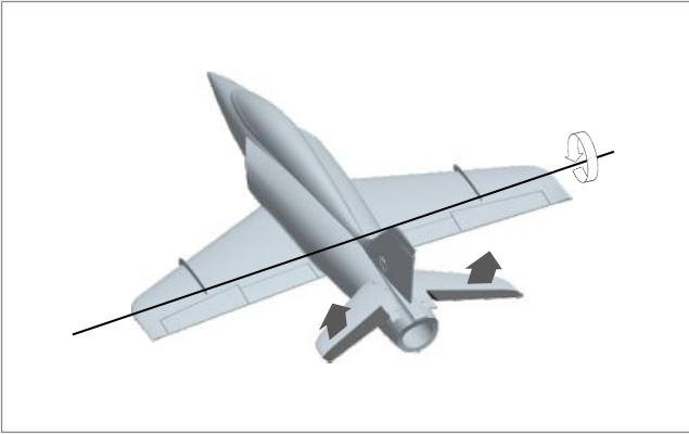
Nose down during flight—Elevator correction diagram
